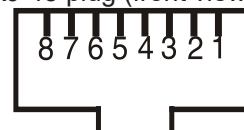
RJ-45 plug (front view):
