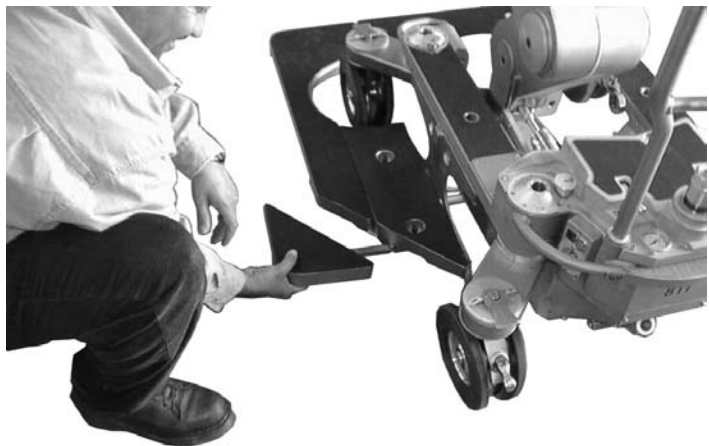
Left Rear Extension Board #1662
