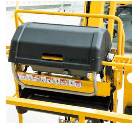
Control box protected by high-strength composite housing
