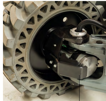
Thick protection shields around traction motors
