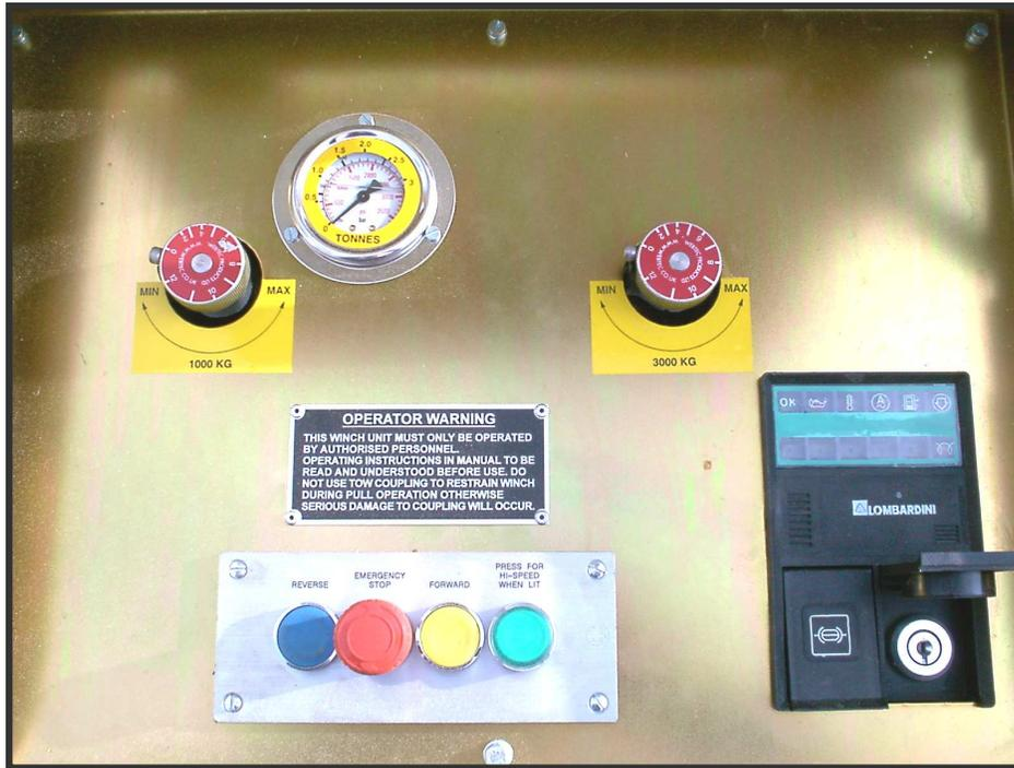
If the left-hand control only is used, the winch will only achieve a maximum line pull of up to 1000 Kg at high speed. If the pull exceeds 1000 Kg, the winch will stop automatically and hold load.
